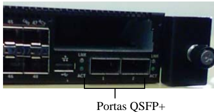
Figura 1. Painel frontal do Dell Networking N4000
