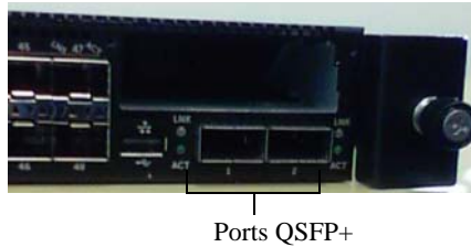
Figure 1. Dell Networking N4000 Panneau avant
