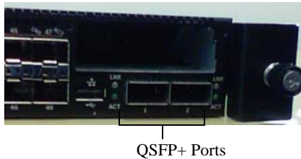
Figure 1. Dell Networking N4000 Front Panel
